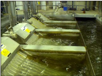
Pictures of Salsnes SFK channel-mounted units at fish farms.
