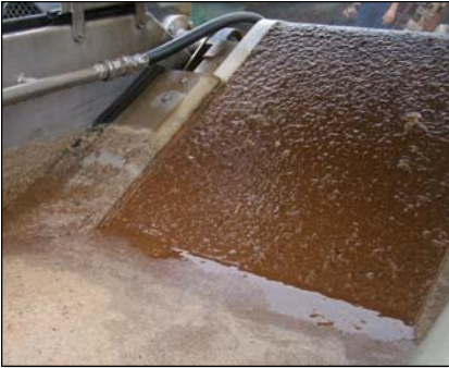
The Salsnes Filter can remove solids as fine as 15-30 microns. The mesh size can be varied depending on the application.
