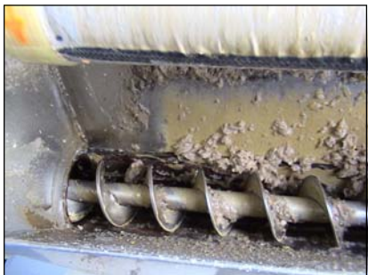
In the hopper, a screw press dewateres the solids. Cake from beef processing facilities is typically 20-25% solids.
