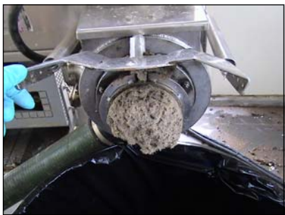
The integrated dewatering feature allows multiple options for disposal of the screenings.
